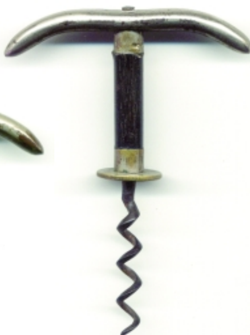
Steel handle and black painted wooden casing
